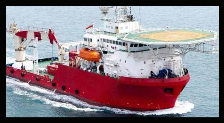
DSV Aureus is a multipurpose worldwide offshore construction, maintenance and diving support vessel, equipped with fully redundant dynamic positioning system, saturation and surface supplied diving systems, helideck and a 50 ton Active heave compensated crane. The vessel can accommodate up to 120 personnel and is SPS compliant.
