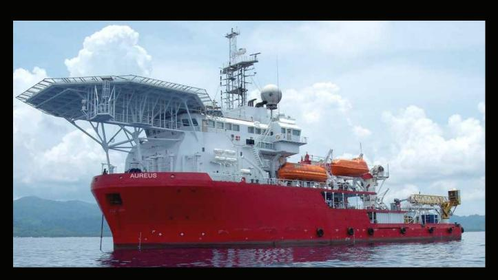
DSV Aureus is a multipurpose worldwide offshore construction, maintenance and diving support vessel, equipped with fully redundant dynamic positioning system, saturation and surface supplied diving systems, helideck and a 50 ton Active heave compensated crane. The vessel can accommodate up to 120 personnel and is SPS compliant.
