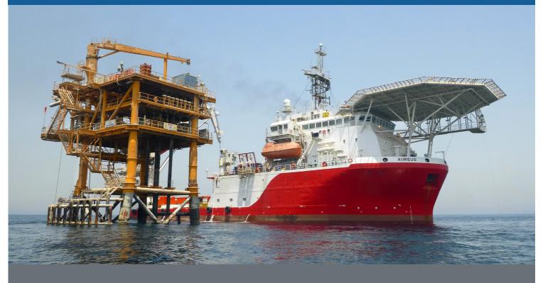
DSV Aureus is a multipurpose worldwide offshore construction, maintenance and diving support vessel, equipped with fully redundant dynamic positioning system, saturation and surface supplied diving systems, helideck and a 50 ton Active heave compensated crane. The vessel can accommodate up to 120 personnel and is SPS compliant.
