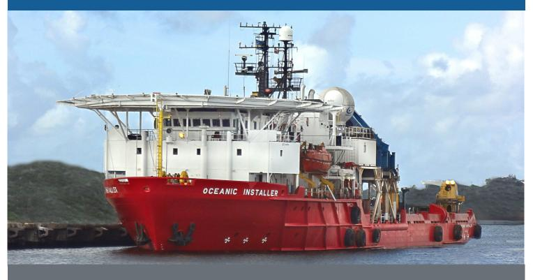
The DSV "OCEANIC INSTALLER" is a multipurpose worldwide offshore construction, maintenance and diving support vessel, equipped with a passive stabilising system, fully redundant dynamic positioning system, saturation and surface supplied diving systems, heavy lifting equipment and helideck.
